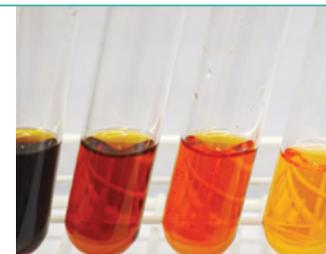
**Fig 6** Use of the phenol-sulphuric test for carbohydrates (sensitivity ~ 10 µg/ml)
