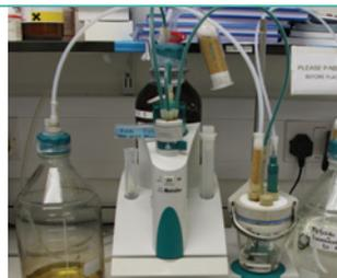
**Fig 5** Karl Fischer apparatus for moisture determination
