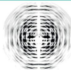
Fig 36 X-Ray diffraction diagram of cellulose
