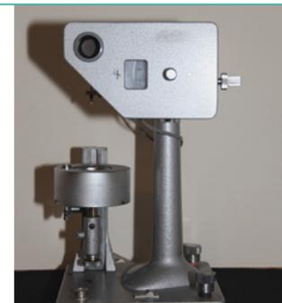
Fig 33 Kruss tensiometer
