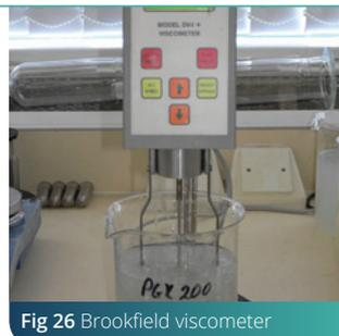
Fig 26 Brookfield viscometer
